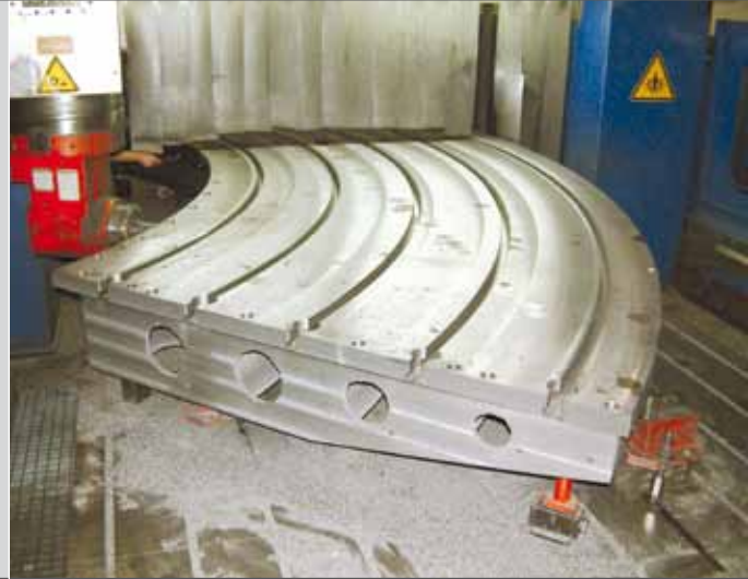
Segment of rotary table with a diameter of 9.000 mm
