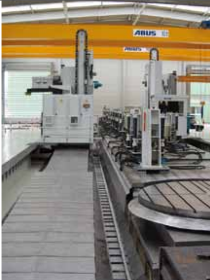
36.000 mm plate field with integrated rotary table for a CNC plate drilling machine
