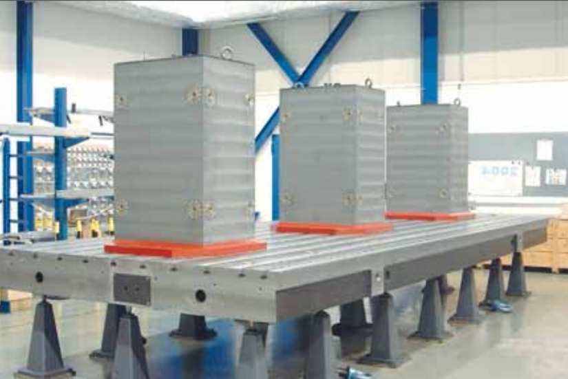
Clamping towers with a zero-point clamping system
