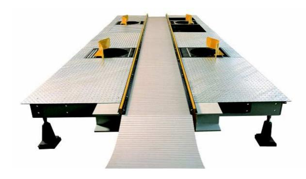
We supply individually designed steel floor covers for different kinds of test rigs. In the steel cover a passable moving floor for the track width and wheelbase is integrated. The cover of the inspection walkway is realized by using a motorized aluminium shutter.
